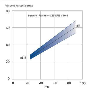
measurements of ferrite in duplex stainless welds. Electronic instruments based on magnetic response, e.g., the Fischer Feritscope, is useful for quality control when adequately calibrated.
