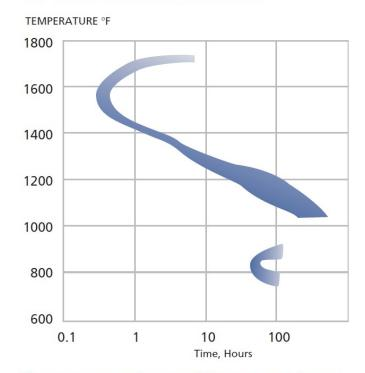
The curve corresponds to an ambient temperature impact toughness of 20 ft.-lb. (27J).
